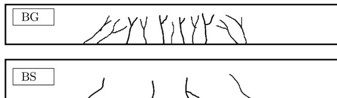
Fig. 9. Diagram of the cracking of beams
