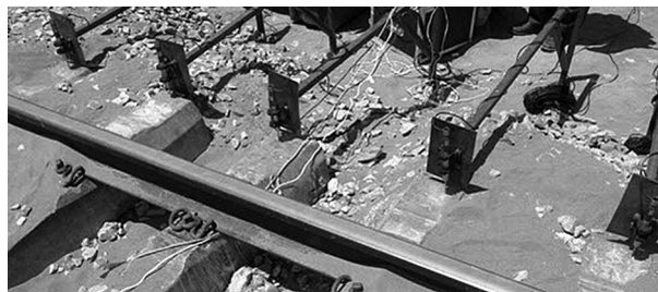
Fig. 6. Linear variable differential transformer (LVDT) for measuring the vertical displacement of the railway track
