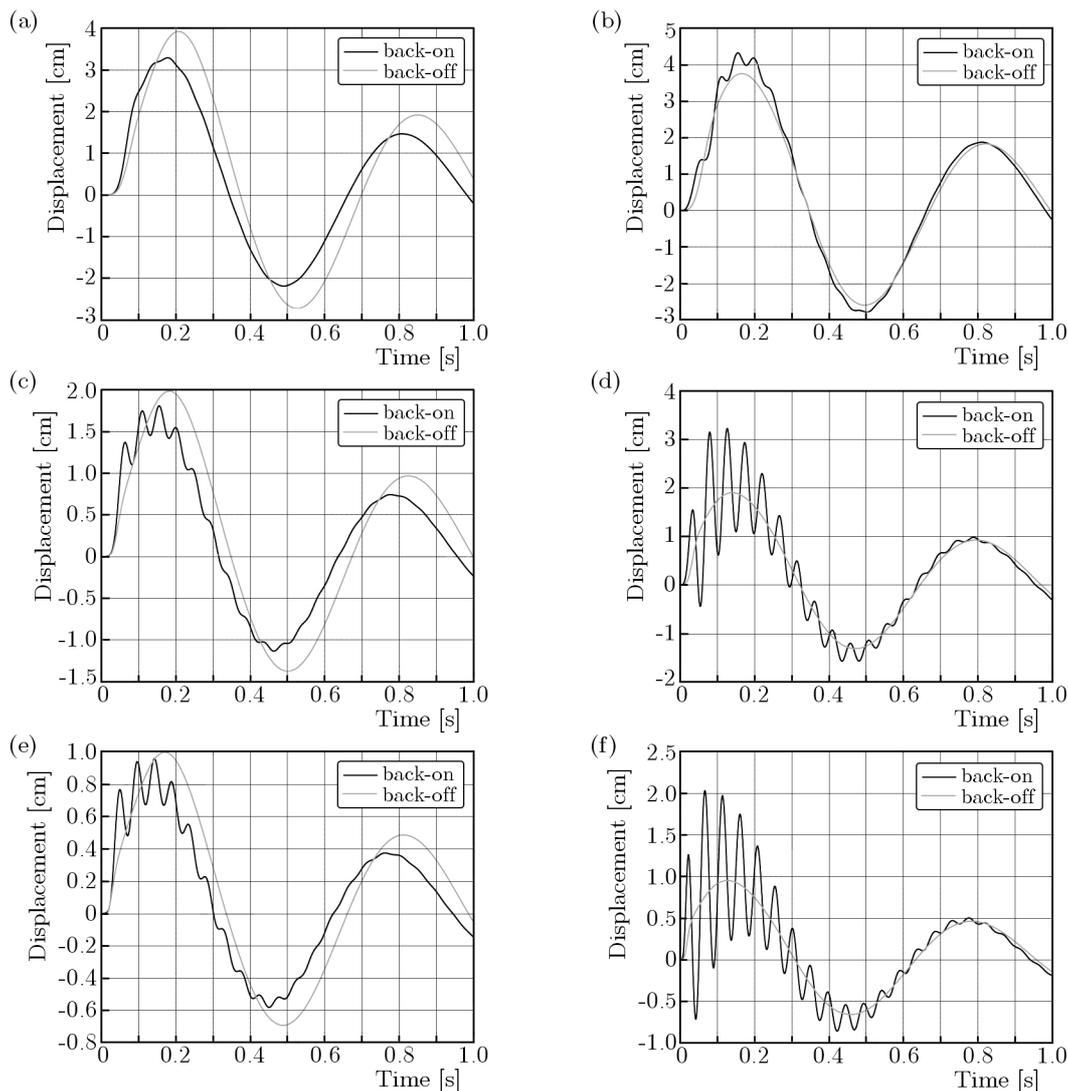
Fig. 5. Response of the human body-seat model with the passive seat to the impulse excitation of amplitude  $h$  equal to 10 cm but different time lengths  $\Delta t$ : (a) upper mass,  $\Delta t = 0.1$  s; (b) lower mass,  $\Delta t = 0.1$  s; (c) upper mass,  $\Delta t = 0.05$  s; (d) lower mass  $\Delta t = 0.05$  s; (e) upper mass,  $\Delta t = 0.025$  s; (f) lower mass,  $\Delta t = 0.025$  s
