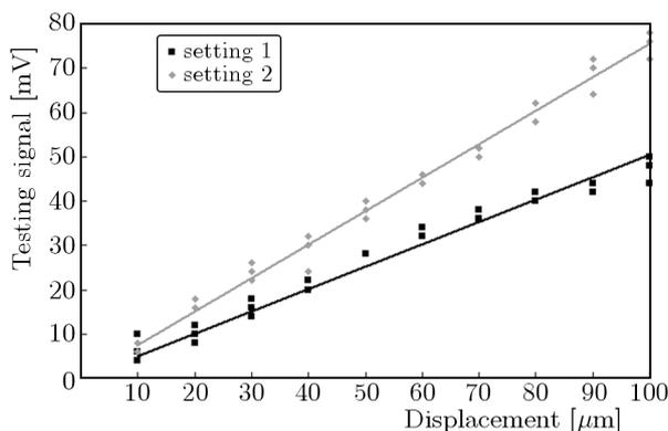
Fig. 5. 5: Sample calibration results for two different testing probe settings ( $x$  axis – displacement in  $\mu\text{m}$ ,  $y$  axis – testing signal in mV)
