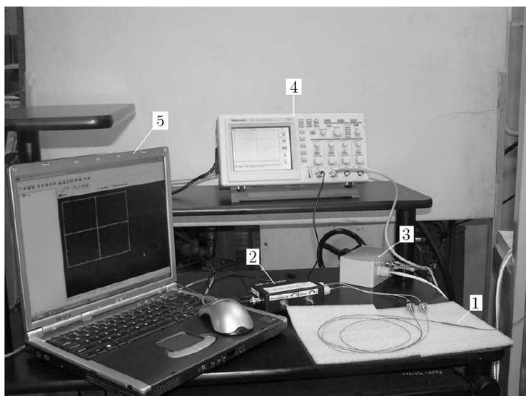
Fig. 8. The measuring system for the micro valve closing element displacement
