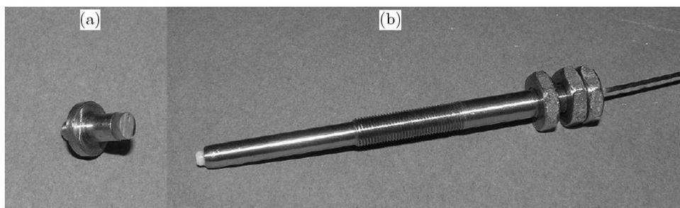
Fig. 3. Cooperating elements: (a) mirror-equipped element whose movements are measured, (b) testing probe with optical fiber installed in its core
