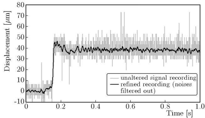
Fig. 9. Exemplary course of the micro valve closing element displacements during a step change in the flow directed at the valve – unaltered signal recording and refined recording (noises filtered out)
