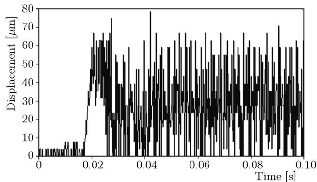
Fig. 10. Exemplary course of the micro valve closing element displacement during a step change in the flow directed at the valve – unstable valve action
