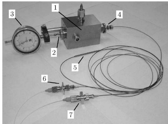
Fig. 4. Studied micro valve during calibration: 1 – micro valve body, 2 – calibration shaft for displacing the closing element, 3 – micrometer gauge for measuring closing element displacements in relation to seat, 4 – testing probe (measuring shaft) containing optical fiber, 5 – fiberoptic coupler, 6 and 7 – coupler-transmitter and coupler-receiver connectors
