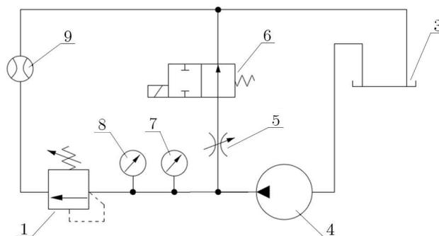
Fig. 7. Diagram of the hydraulic system for measurements of the micro valve closing element displacement
