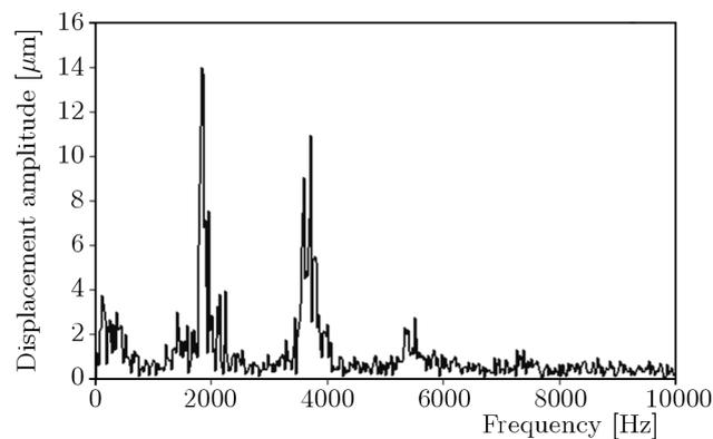
Fig. 11. Exemplary valve vibration frequency analysis during an unstable action
