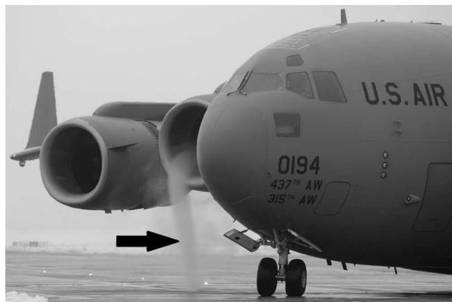
Fig. 1. Vortex (marked with an arrow) in the inlet system of the F117-PW-100 (PW2040) engine on a C-17 aircraft
