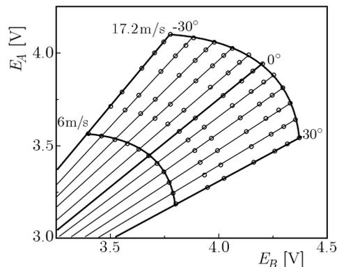
Fig. 1. Calibration results showing calibration points (o), constant flow velocity lines and constant yaw angle lines determined from the calibration points
