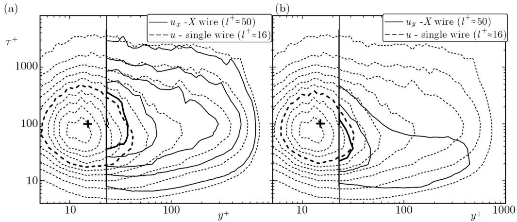
Fig. 4. Iso-contours of the energy spectra  $E/u_\tau^2$ : effect of the length scale and geometry of the probe: single-wire  $l^+ = 16$  (solid); X-wire  $l^+ = 50$  (dashed) on streamwise energy (a) and comparison of the streamwise single-wire and wall-normal X-wire energy (b). Contours are from 0 to 2 with the steps equal 0.2
