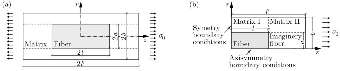
Fig. 1. (a) Micromechanical unit cell. (b) Axi-symmetric model
