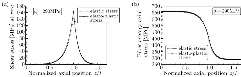
Fig. 4. Shear stress at  $r = a$  (a) and fiber average axial stress (b) for  $\sigma_0 = 290$  MPa
