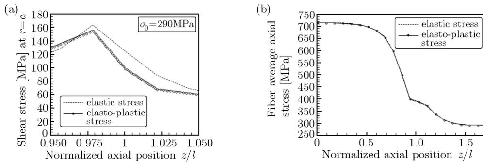
Fig. 9. Numerical results – shear stress at  $r = a$  (a) and fiber average axial stress (b) for  $\sigma_0 = 290$  MPa
