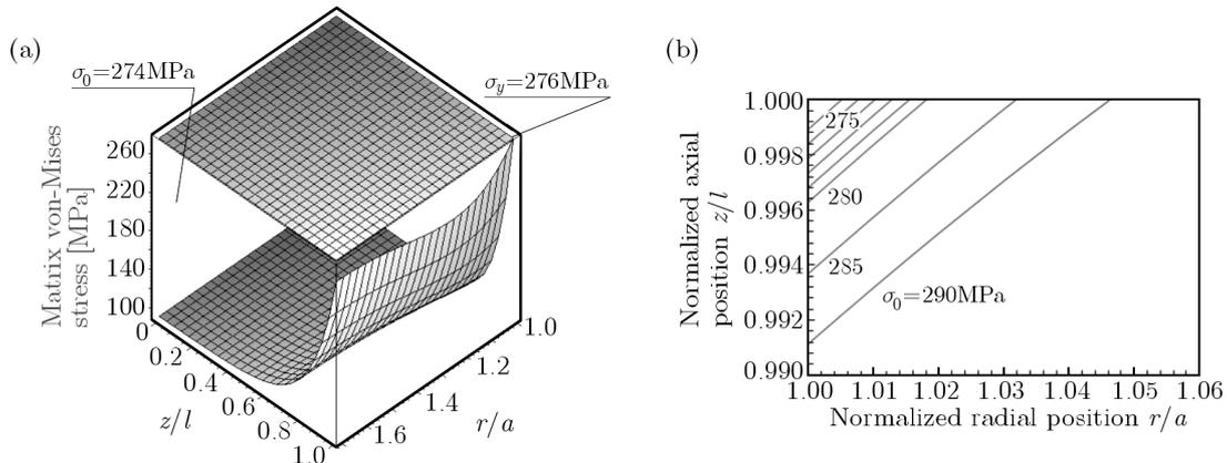
Fig. 2. (a) Matrix equivalent stress for  $\sigma_0 = 274$  MPa, (b) expansion of the plastic region in the matrix model
