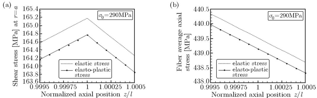
Fig. 5. Shear stress at  $r = a$  (a) and fiber average axial stress (b) for  $\sigma_0 = 290$  MPa
