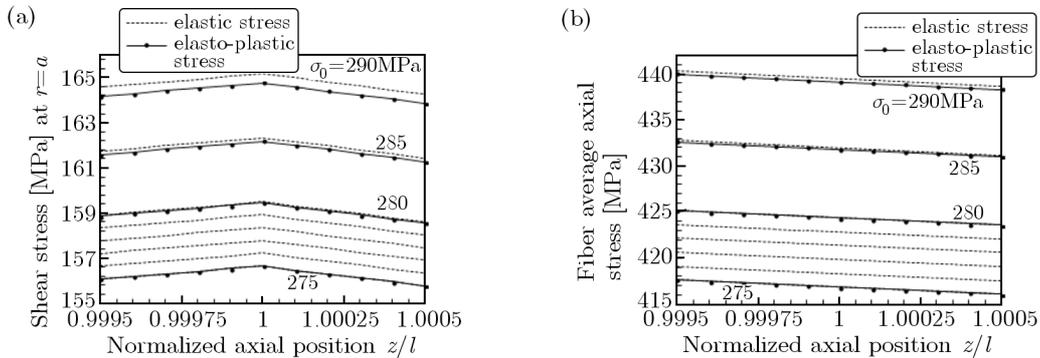
Fig. 6. Shear stress at  $r = a$  (a) and fiber average axial stress (b), different loadings  $\sigma_0$
