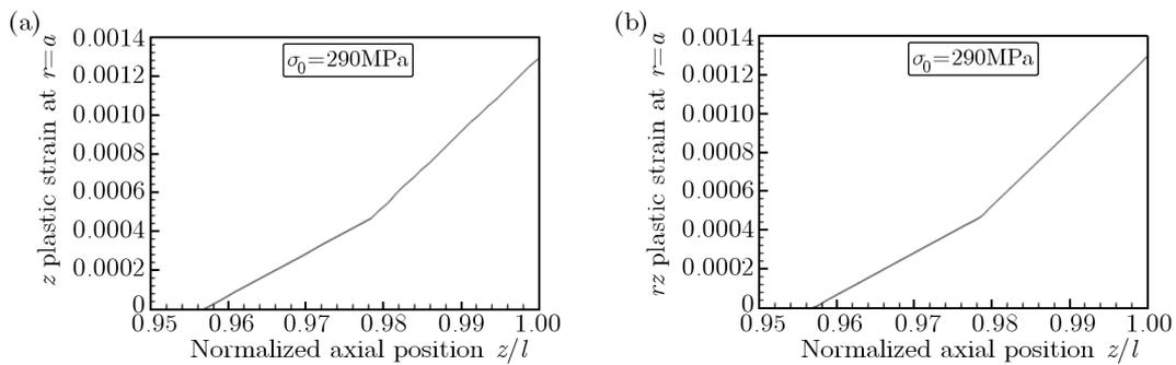
Fig. 8. Numerical results –  $\epsilon_z^p(a, z)$  at: (a)  $r = a$  and (b)  $r = a$
