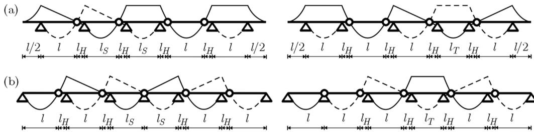
Fig. 10. Optimal beams with a different number of supports and equal values of the absolute maximum moment: (a) two topologies from the class  $\mathbf{T}_2^6$ , (b) two topologies from the class  $\mathbf{T}_{44}^7$
