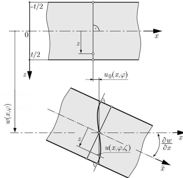
Fig. 3. Deformation of the plane cross section scheme
