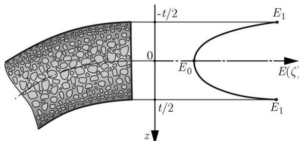
Fig. 2. Scheme of a porous-cellular shell structure
