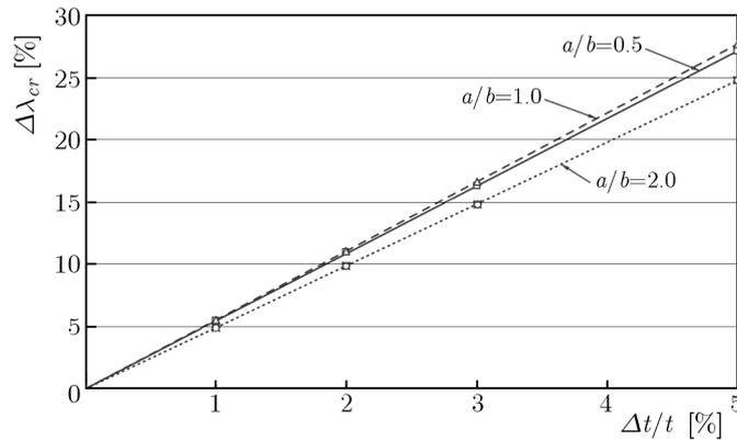
Fig. 2. Relative change of the buckling load factor ( $\Delta\lambda_{cr}$  [%]) for different  $a/b$  aspect ratios and tolerance levels  $\Delta t/t$ . The results are calculated with respect to the nominal (ideal) solution
