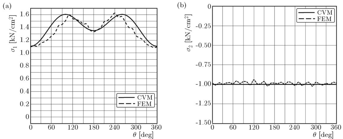
Fig. 8. Comparative diagram of the stress  $\sigma_1$  (a) and  $\sigma_2$  (b) at the contour of the eccentric hole
