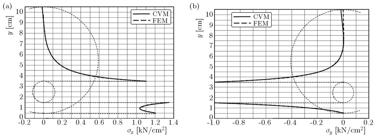
Fig. 9. Comparative diagram of the stress  $\sigma_x$  (a) and  $\sigma_y$  (b) at the intersection of the  $y$  axis
