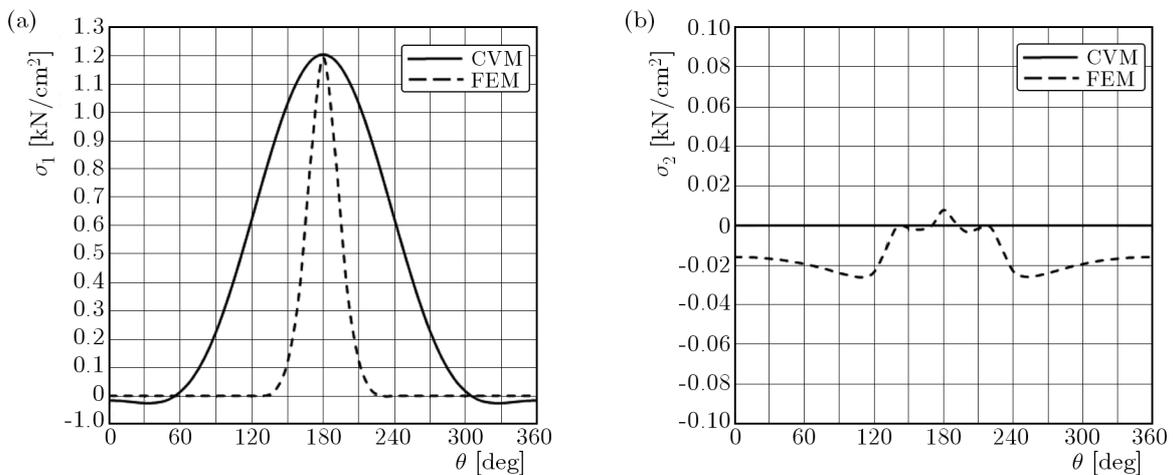
Fig. 7. Comparative diagram of the stress  $\sigma_1$  (a) and  $\sigma_2$  (b) at the outer contour of the disc
