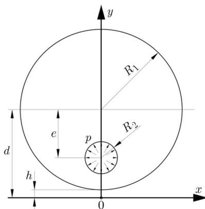
Fig. 3. The disc weakened by an eccentric circular hole
