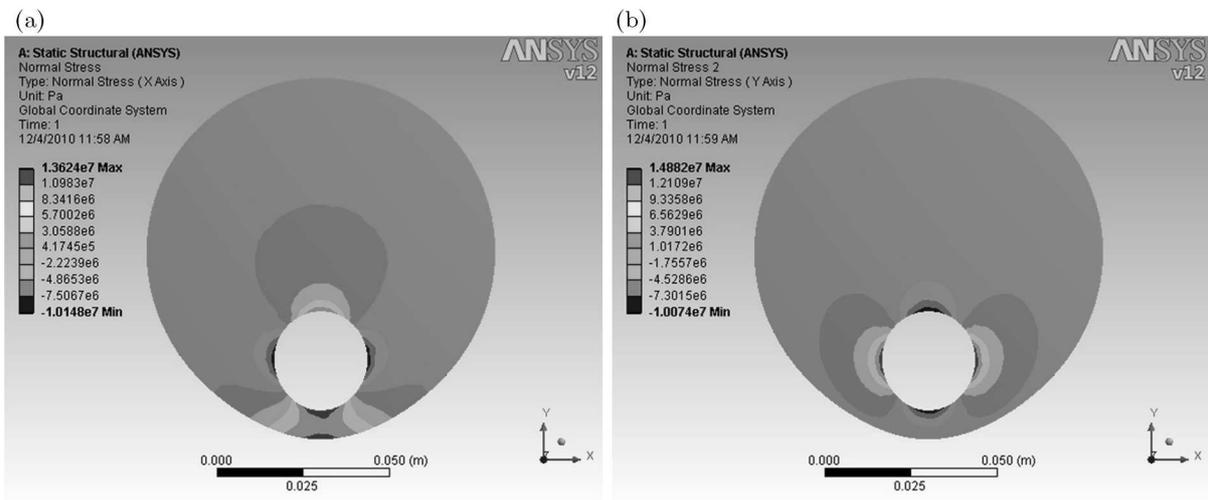
Fig. 5. Normal stress  $\sigma_x$  (a) and  $\sigma_y$  (b)
