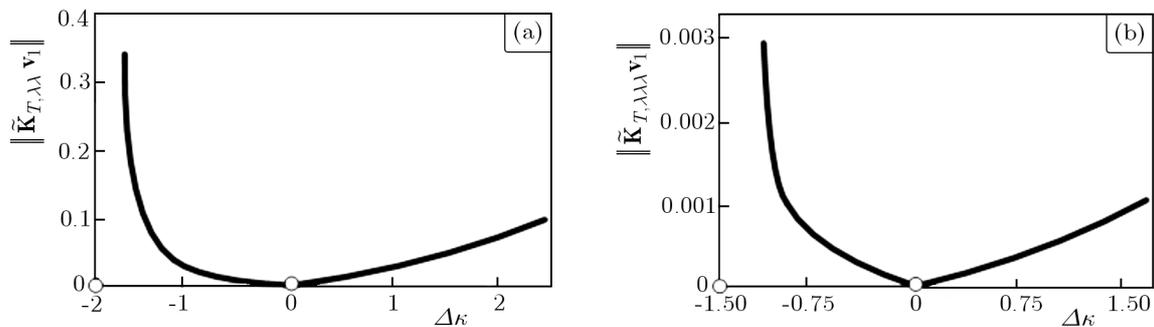
Fig. 5. Sensitivity analysis of bifurcation buckling of a family of two-hinged arches: (a)  $\|\tilde{\mathbf{K}}_{T,\lambda\lambda}\mathbf{v}_1\|_2$  and (b)  $\|\tilde{\mathbf{K}}_{T,\lambda\lambda\lambda}\mathbf{v}_1\|_2$  as functions of  $\Delta\kappa$  representing the deviation from a thrust-line arch (Mang and Höfinger, 2012)
