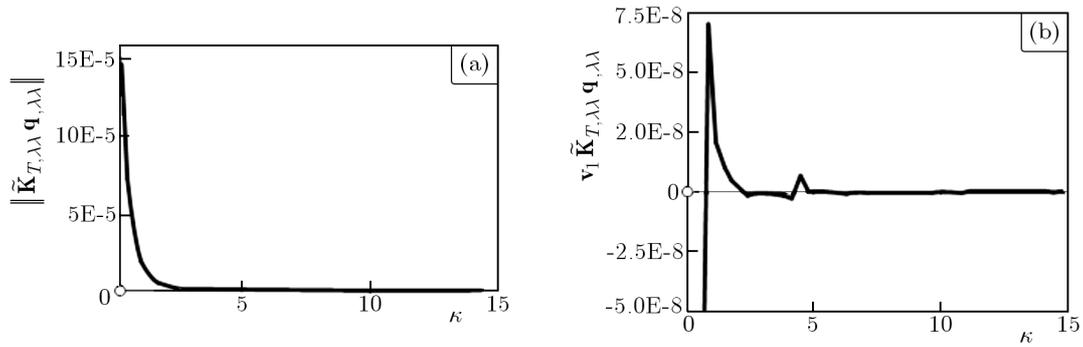
Fig. 6. Sensitivity analysis of bifurcation buckling of a *von Mises* truss with an elastic spring attached to the load point: (a)  $\|\tilde{\mathbf{K}}_{T,\lambda\lambda} \mathbf{q}_{,\lambda\lambda}\|_2$  and (b)  $\mathbf{v}_1 \tilde{\mathbf{K}}_{T,\lambda\lambda} \mathbf{q}_{,\lambda\lambda}$  as functions of the scaling parameter  $\kappa$  of the spring stiffness (Höfinger, 2010)
