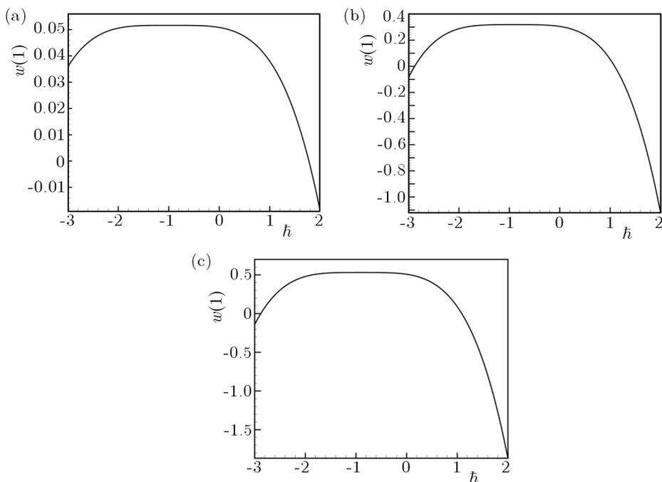
Fig. 1.  $\hbar$ -curves with the 6-th order approximation showing the convergence of HAM results;  $w$  is the deflection of the beam at a desired point versus  $\hbar$ , which indicates the region where the results converge; (a)  $\beta = 5, \delta = 0.1, \mu = 1$ , (b)  $\beta = 6, \delta = 0.6, \mu = 0.5$ , (c)  $\beta = 10, \delta = 1, \mu = 0.3$
