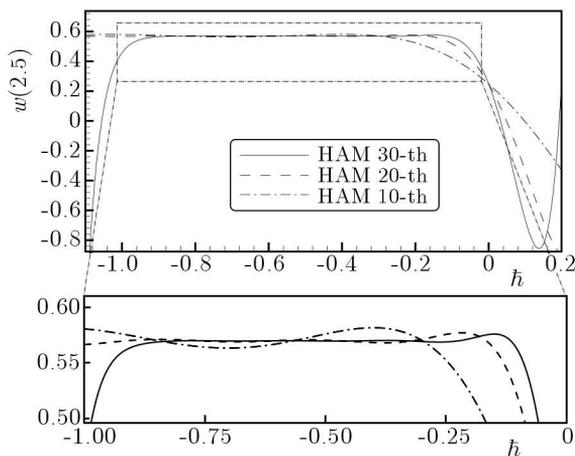
Fig. 3.  $\hbar$ -curve indicating the convergence of HAM results with respect to the order of HAM method and various values of  $\hbar$ .  $w$  shows the deflection of the beam at  $\xi = 2.5$
