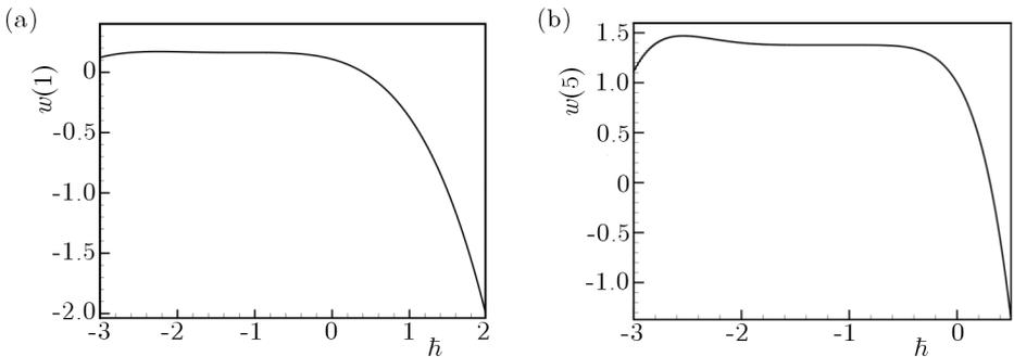
Fig. 2.  $\hbar$ -curves with the 6-th order approximation showing the convergence of HAM results;  $w$  is the deflection of the beam at a desired point versus  $\hbar$ , which indicates the region where the results converge; (a)  $\beta = 5$ ,  $\bar{P}/k = 1$ ,  $\mu = 1$ ,  $\alpha = 2.5$ ,
