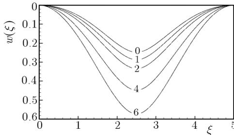
Fig. 4. Deflection of the clamped-clamped beam obtained by the HAM method with respect to various values of  $\mu$ ;  $\beta = 5$ ,  $\bar{P}/k = 0.5$ ,  $\alpha = 2.5$
