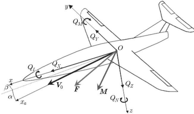
Fig. 3. Vectors of force and the moment of the external force as well as their components in the reference system  $Oxyz$
