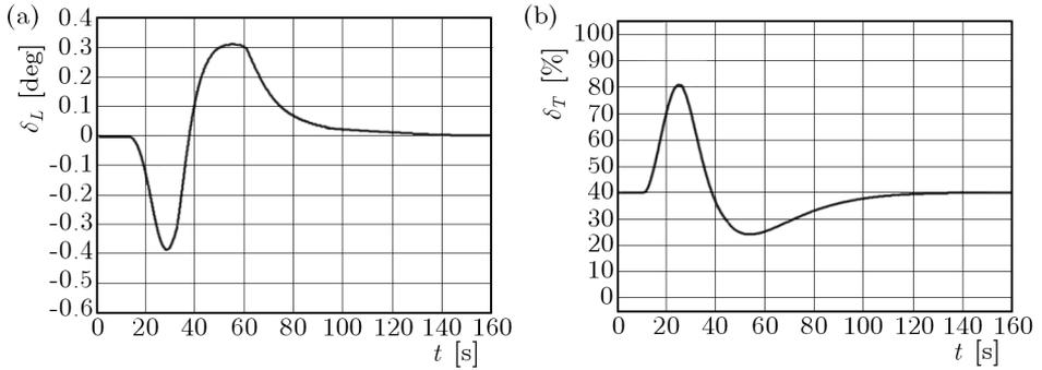
Fig. 8. History of the aileron deflection (a) and the changing engine thrust (b)
