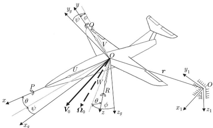
Fig. 2. Adopted reference systems, linear and angular speed of a UAV
