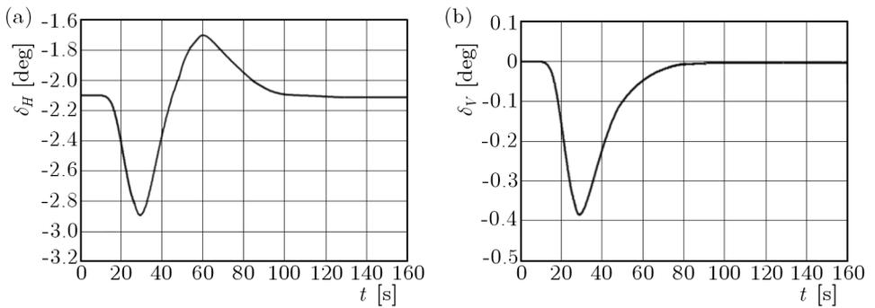
Fig. 7. History of the elevator (a) and rudder (b) deflection
