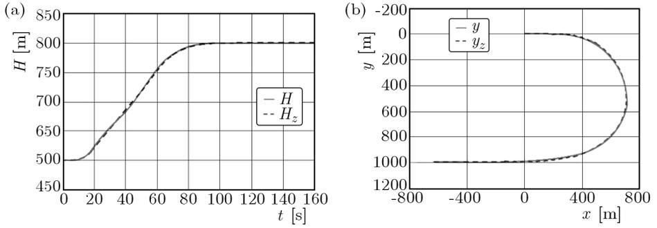
Fig. 5. Diagrams of the real and preset UAV flight altitudes (a) and lateral projections (b)
