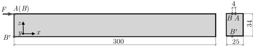
Fig. 2. Geometric configuration of the steel beam [mm]
