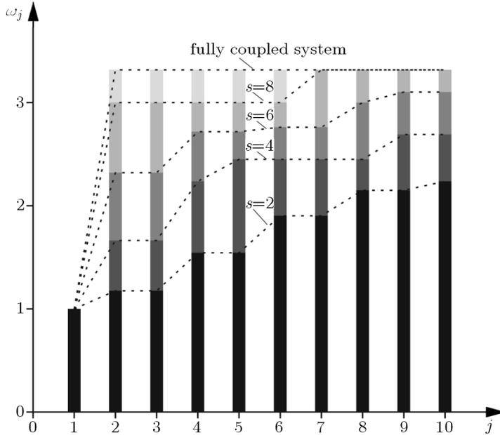
Fig. 2. Spectra of natural frequencies of the regular system consisting of 10 masses for 5 different degree of coupling, for  $m = 1$  kg and  $k = p = 1$  N/m
