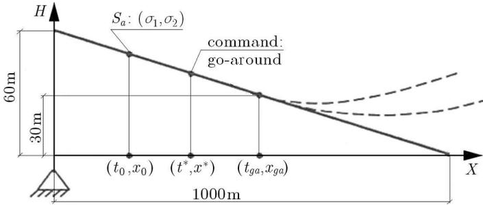
Fig. 2. Final phase of aircraft approach
