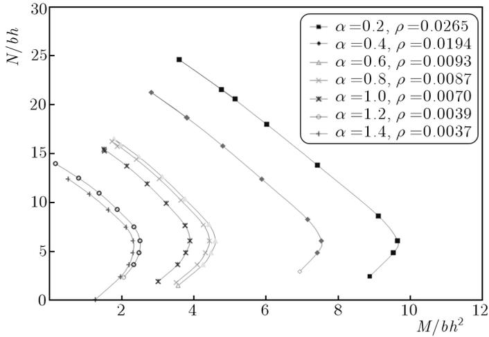
Fig. 4. Interaction curves at  $d/h = 0.9$  and  $\beta = 4.5$
