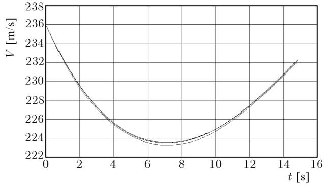
Fig. 5. Speed of the bomb flight
