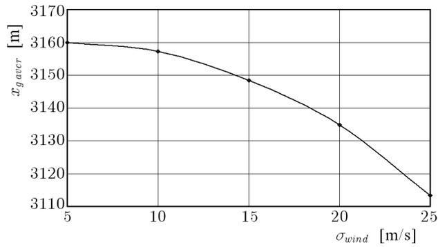
Fig. 9. Average value of  $x_g$  coordinate of the point of impact
