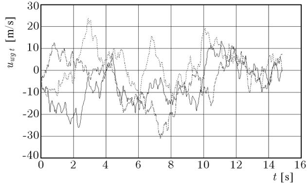
Fig. 2. Diagram of wind component  $u_{wgt}$  versus time
