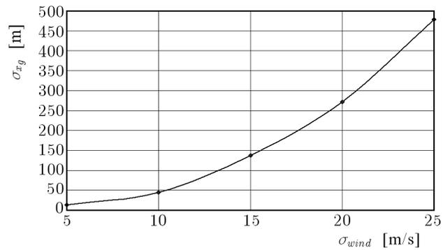
Fig. 10. Standard deviation of  $x_g$  coordinate of the point of impact
