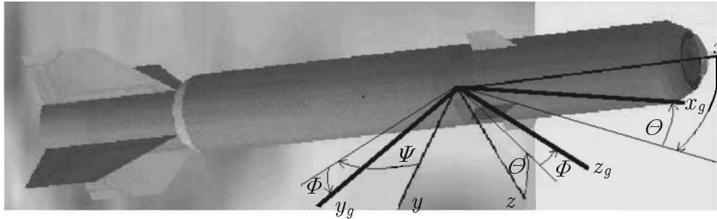
Fig. 1. Systems of coordinates with angles of transition
