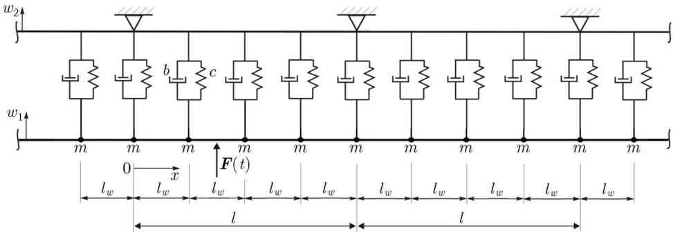
Fig. 1. Physical model of the system
