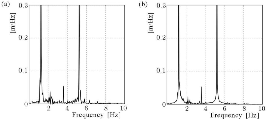
Fig. 2. Amplitude spectrum of displacement at  $x = 8$  m: (a) contact wire, (b) carrying cable
