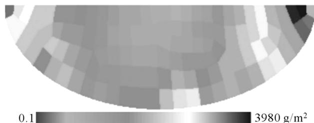
Fig. 22. Total velocity of erosive wear of the wall material used in the dissipative element for the Bitter model of wear
