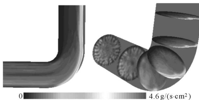
Fig. 11. Concentration distribution for the solid fraction in selected sections of the calculation area without the dispersing element
