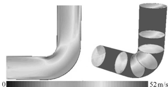
Fig. 7. Gas velocity distributions in selected sections of the calculation area without the dissipative element
