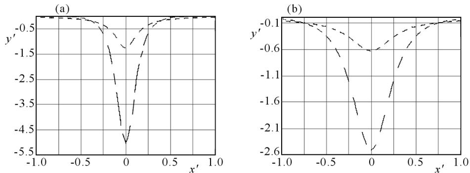
Fig. 4. Lines of constant dimensionless stresses  $\sigma_{yy}^{(j)}(x', y')/\sigma_0$  for  $P = \sigma_0$ ,  $Q = 0$ ; (a)  $y' = 0.25$ , (b)  $y' = 0.5$  ( $E_1/E_2 = 4$ ,  $\eta = 0.25$ ,  $\nu_1 = \nu_2 = 0.3$ ,  $a = 0$ )
