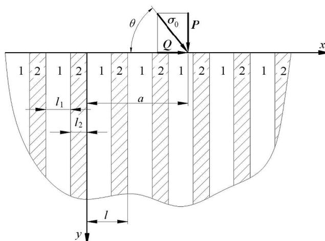
Fig. 1. A cross-section of the periodically laminated half-space
