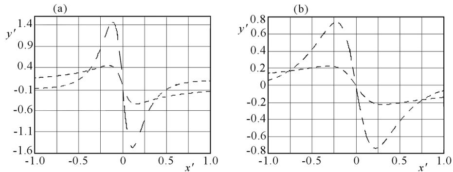
Fig. 5. Lines of constant dimensionless stresses  $\sigma_{yy}^{(j)}(x', y')/\sigma_0$  for  $P = 0$ ,  $Q = \sigma_0$ ; (a)  $y' = 0.25$ , (b)  $y' = 0.5$  ( $E_1/E_2 = 4$ ,  $\eta = 0.25$ ,  $\nu_1 = \nu_2 = 0.3$ ,  $a = 0$ )
