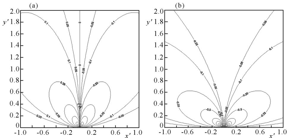
Fig. 3. Lines of constant dimensionless stresses  $\sigma_{xy}^{(j)}(x', y')/\sigma_0$  for two cases: (a)  $P = \sigma_0, Q = 0$ , (b)  $P = 0, Q = \sigma_0$  ( $E_1/E_2 = 4, \eta = 0.5, \nu_1 = \nu_2 = 0.3, a = 0$ )
