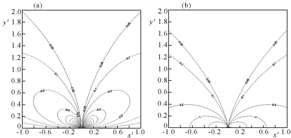
Fig. 2. Lines of constant dimensionless stresses  $\sigma_{xx}^{(j)}(x', y')/\sigma_0$  for two cases: (a)  $P = \sigma_0, Q = 0$ , (b)  $P = 0, Q = \sigma_0$  ( $E_1/E_2 = 4, \eta = 0.5, \nu_1 = \nu_2 = 0.3, a = 0$ )
