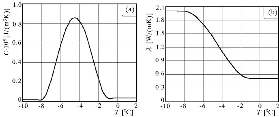
Fig. 2. (a) Substitute thermal capacity; (b) thermal conductivity
