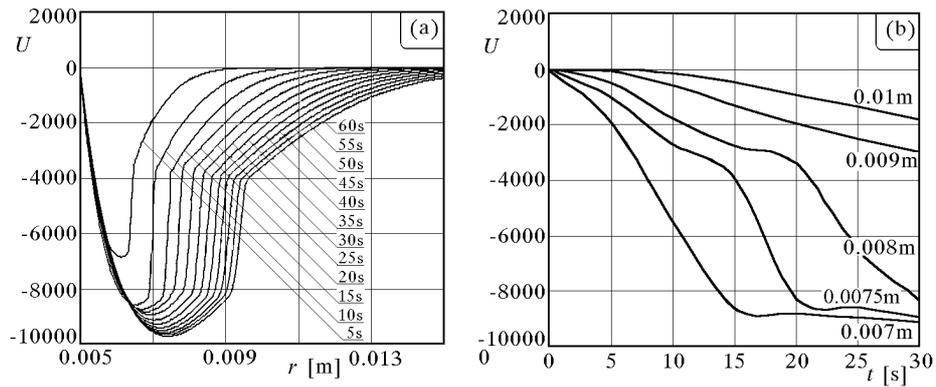
Fig. 5. (a) Distribution of the function  $U = DV/Db$ ; (b) courses of the function  $U$  at selected points
