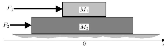
Fig. 5. Two-mass system with two friction forces;  $M_1, M_2$  – masses of blocks,  $F_1, F_2$  – external forces,  $F_{T12}, F_{T20}$  – friction forces,  $F_{T012}, F_{T020}$  – maximal dry friction forces,  $C_{12}, C_{20}$  – damping factors
