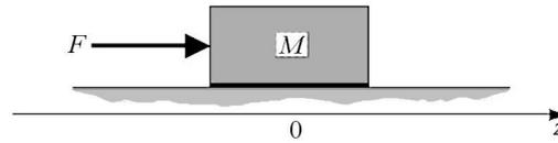
Fig. 3. Single-mass system with friction;  $M$  – mass,  $F$  – external acting force (notation of friction parameters in accordance with Fig. 1)
