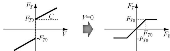
Fig. 1. Typical piecewise linear friction force characteristics:  $F_T(V)$  – Coulomb-like kinetic friction characteristic,  $F_T(F_W)$  – saturation static friction characteristics.
