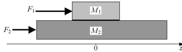
Fig. 4. Two-mass system with single friction;  $M_1, M_2$  – masses of blocks,  $F_1, F_2$  – external forces,  $F_{T12}$  – friction force,  $F_{T012}$  – maximum dry friction force,  $C_{12}$  – damping factor
