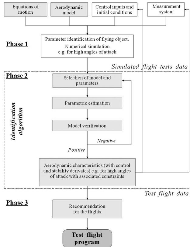
Fig. 2. Phases of practical identification of aerodynamic characteristics of a flying object (Giergiel and Uhl, 1990; Goszczyński, 2000)
