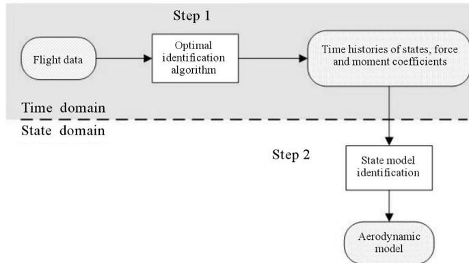
Fig. 6. Overview of the Estimation Before Modelling technique (Stalford, 1979)
