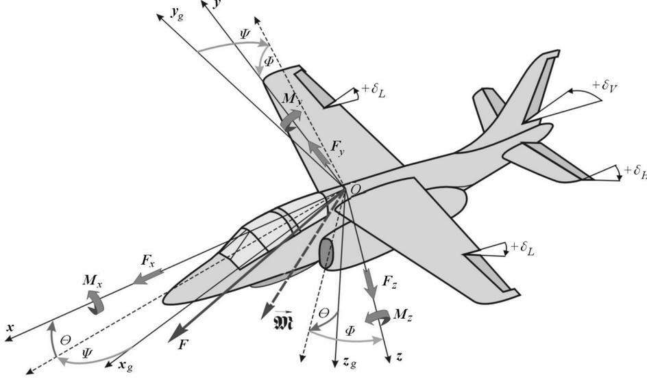
Fig. 3. Assumed FO co-ordinate systems and displacements of control surfaces
