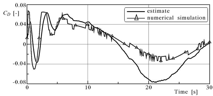
Fig. 11. Estimation history of the aerodynamic drag coefficient  $C_D = f(t)$  (EBM)
