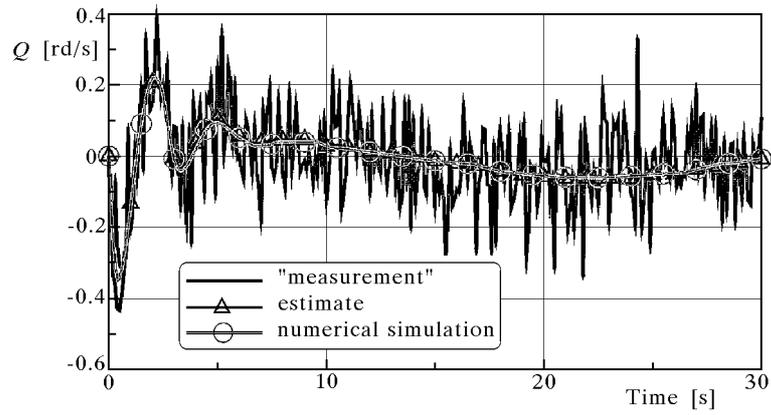
Fig. 10. History of the pitch angular velocity  $Q$  (EBM)
