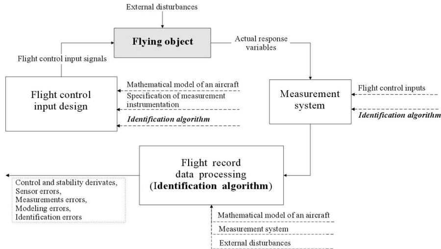
Fig. 1. Correlation in the process of identification of aerodynamic characteristics
