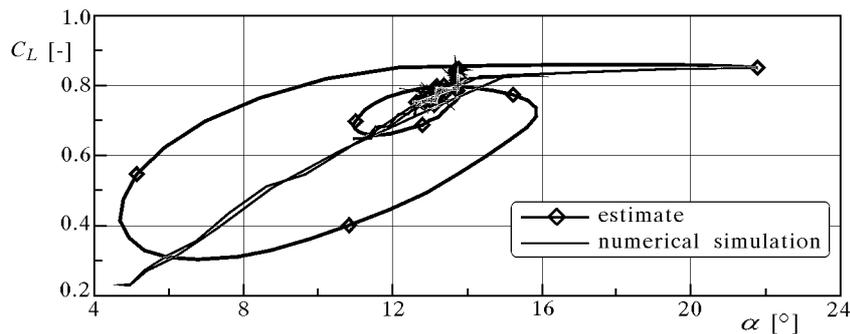
Fig. 13. Estimation of the aerodynamic lift coefficient  $C_L = f(\alpha)$  (EBM)
