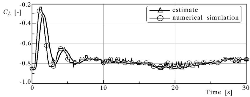
Fig. 12. Estimation history of the aerodynamic lift coefficient  $C_L = f(t)$  (EBM)
