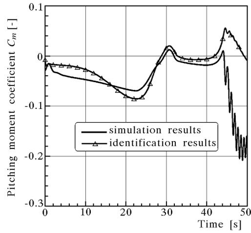
Fig. 5. Identification of the pitching moment coefficient  $C_m$  (FN)
