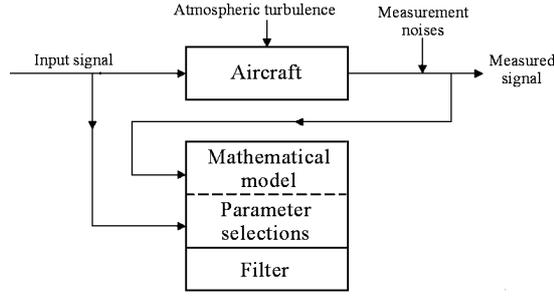
Fig. 7. Concept of the EBM method (Goszczyński *et al.*, 2000)
