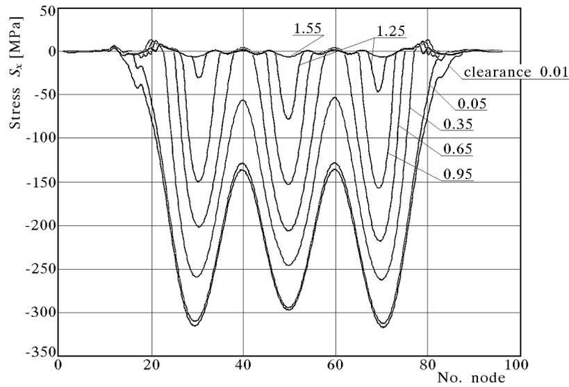
Fig. 7. The effect of clearance size upon the stress  $S_x$
