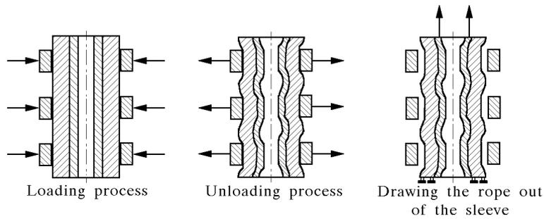
Fig. 3. Scheme of the mounting process
