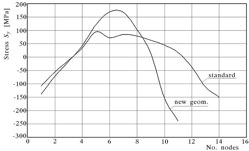
Fig. 12.  $S_y$  stress in the basic and variable-diameter joints
