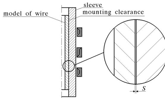
Fig. 2. Scheme of the necessary mounting clearance
