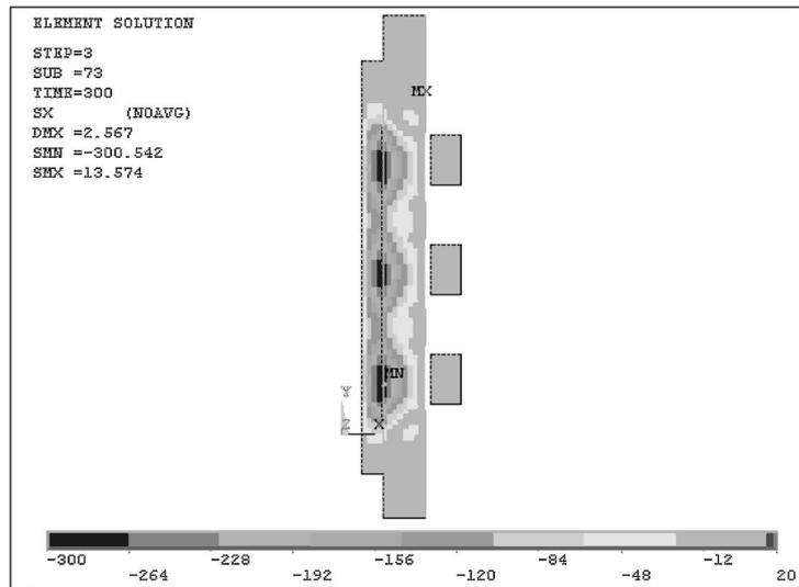
Fig. 5.  $S_x$  stress in the basic variant of the joint
