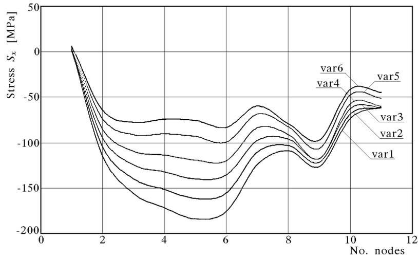
Fig. 14. Courses of the  $S_x$  stress in different variants of the joint geometry
