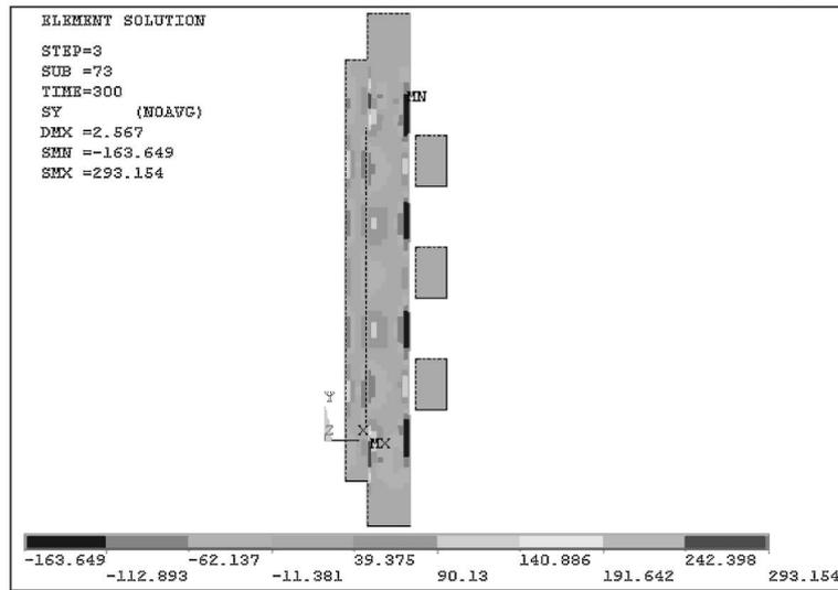
Fig. 6.  $S_y$  stress in the basic variant of the joint
