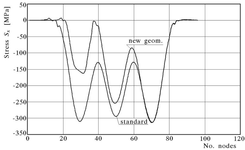
Fig. 11.  $S_x$  stress in the basic joint and in the joint with the variable external diameter
