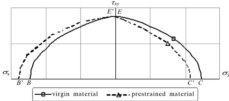
Fig. 6. Ellipses  $BEC$  and  $B'E'C'$  –  $D0$  direction view (assumption)
