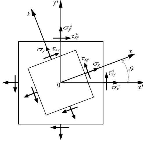
Fig. 1. The fatigue stress distribution in the elementary area
