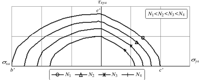
Fig. 8. Ellipses  $b'e'c'$  for different fatigue life –  $D0$  direction view (assumption)
