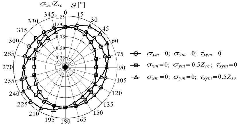
Fig. 2. Dependence of  $\sigma_{xA}$  on the angle  $\vartheta$
