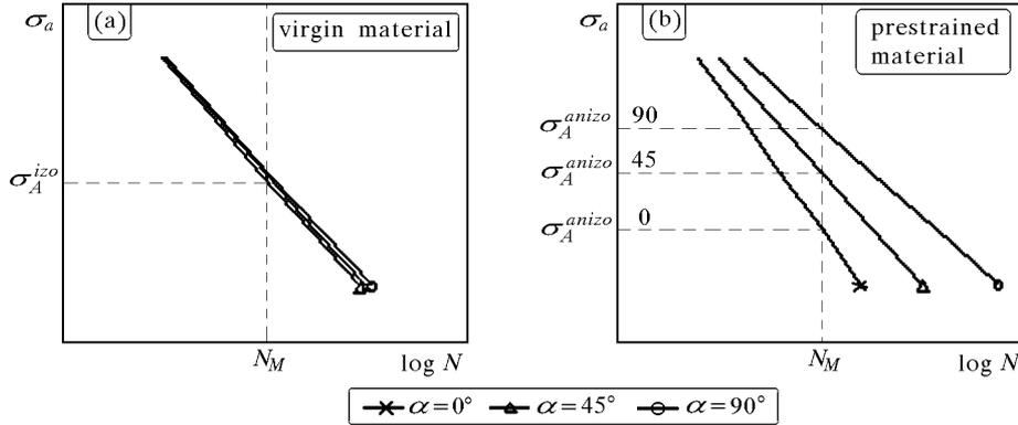
Fig. 9. Wöhler’s lines: (a) virgin material; (b) prestrained material (assumption)
