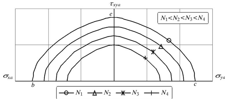
Fig. 7. Ellipses  $bec$  for different fatigue life –  $D0$  direction view (assumption)
