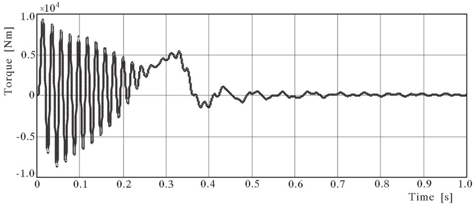
Fig. 10. Electromagnetic torque of the driving motor
