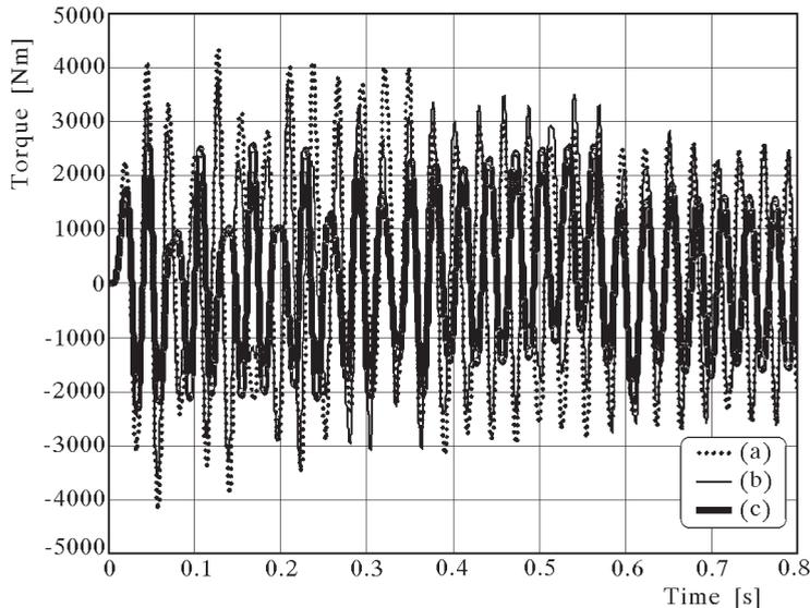
Fig. 16. Torque on the safety shaft (a) before optimization, (b) after optimization of selected parameters of the electric motor ( $L_m, R_r$ ), (c) after optimization of the parameters  $L_m, R_r$  of the electric motor and stiffness of the shaft
