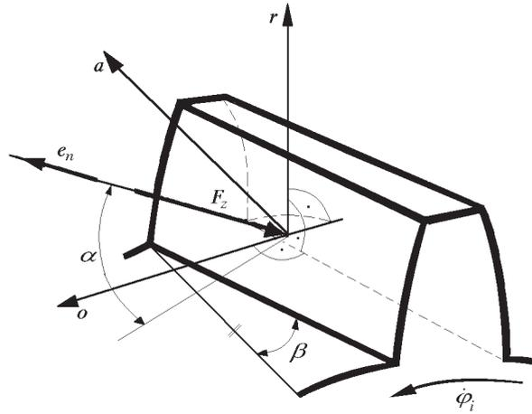
Fig. 5. Forces acting on the tooth of the gear wheel reduced to the contact point
