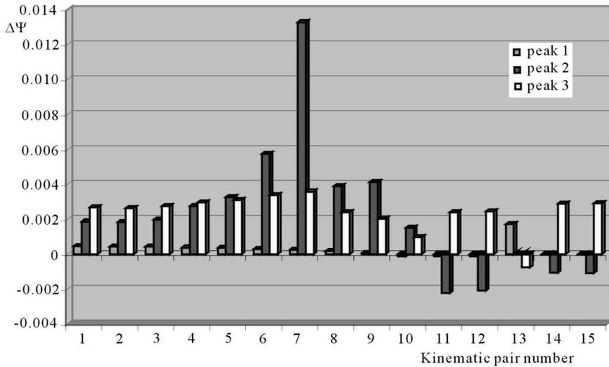
Fig. 12. Influence of the stiffness coefficient of the safety shaft on the peaks of dynamic forces in particular kinematic pairs
