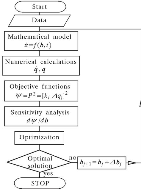
Fig. 1. Block diagram of the algorithm of optimization of the dynamic properties;  $\mathbf{x}$  is the vector of state variables,  $\mathbf{q}$  is the vector of generalized coordinates
