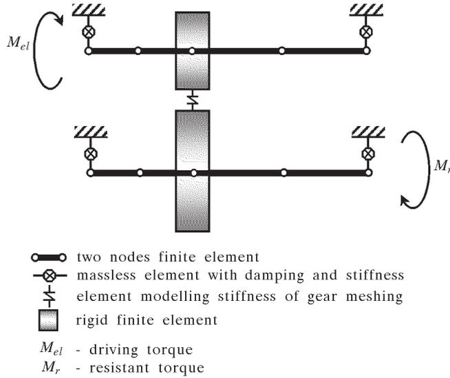
Fig. 3. Physical model of a spur gear pair modelled by the hybrid method
