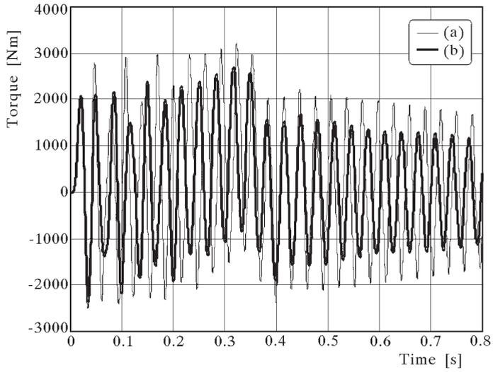
Fig. 13. Dynamic torsional torque in the 1st kinematic pair with the safety shaft (a) before and (b) after optimization
