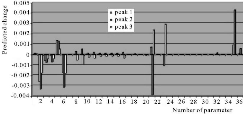
Fig. 15. Relative changes of the peak values of the objective function describing the torque on the output shaft due to an increase in some parameters of the electric (1-5) and mechanical (6-36) parts of the system during the start-up, where: 1 –  $L_m$ , 2 –  $L_s$ , 3 –  $L_r$ , 4 –  $R_s$ , 5 –  $R_r$ , 6-21 – selected mass moments of inertia and masses, 22-36 – selected stiffness coefficients of the shafts, meshes and bearings
