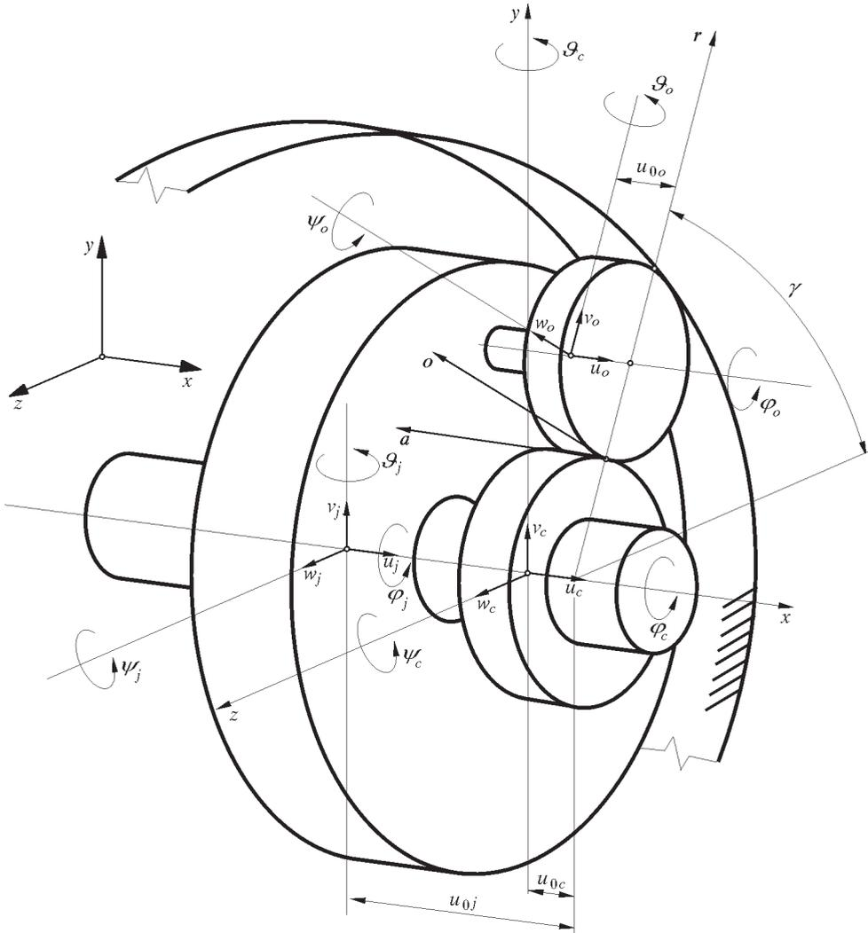
Fig. 6. Model of a planetary gear
