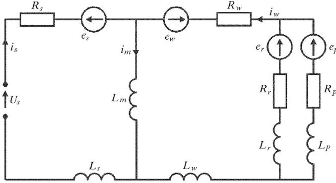
Fig. 2. Circuit model of an inductance motor with two substitute circuits in the rotor;  $e_s$ ,  $e_w$ ,  $e_r$ ,  $e_p$  are rotation voltages in circuits of the stator and rotor
