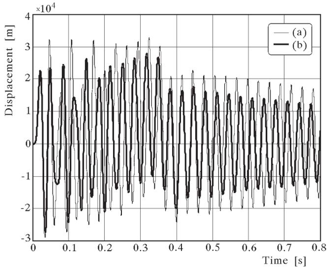
Fig. 14. Displacement of one of the shaft bearings in the direction of the  $x$ -axis (a) before optimization and (b) after optimization
