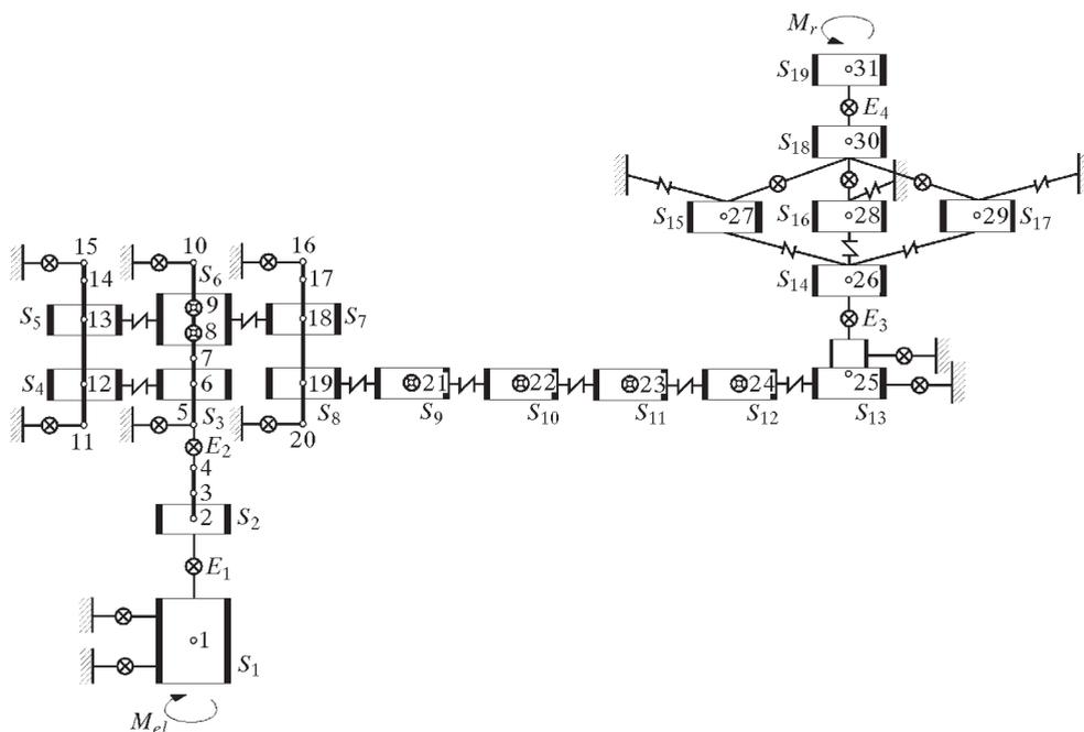
Fig. 7. Dynamical model of transverse torsional vibrations of the transmission system
