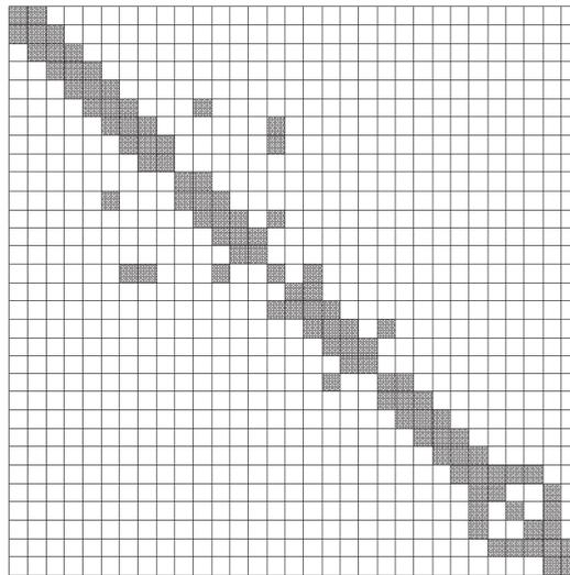
Fig. 9. Nonzero blocks of the stiffness matrix referring to particular nodes of the model
