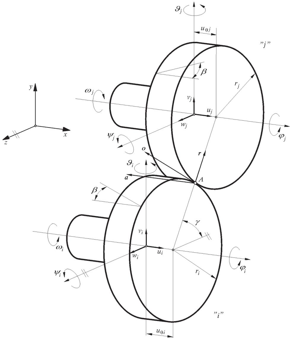
Fig. 4. Single-stage spur gear
