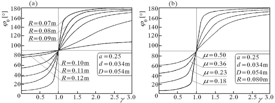
Fig. 5. Pphase displacement angle  $\varphi_0$  as a function of the dimensionless frequency  $\gamma$  for various values: (a) of the external radius  $R$ , (b) of the friction coefficient  $\mu$
