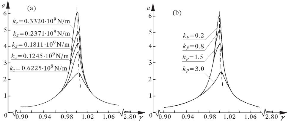
Fig. 4. Resonant curves for various values: (a) of the discs and plunger equivalent rigidity  $k_z$ , (b) of the gain factor  $k_p$
