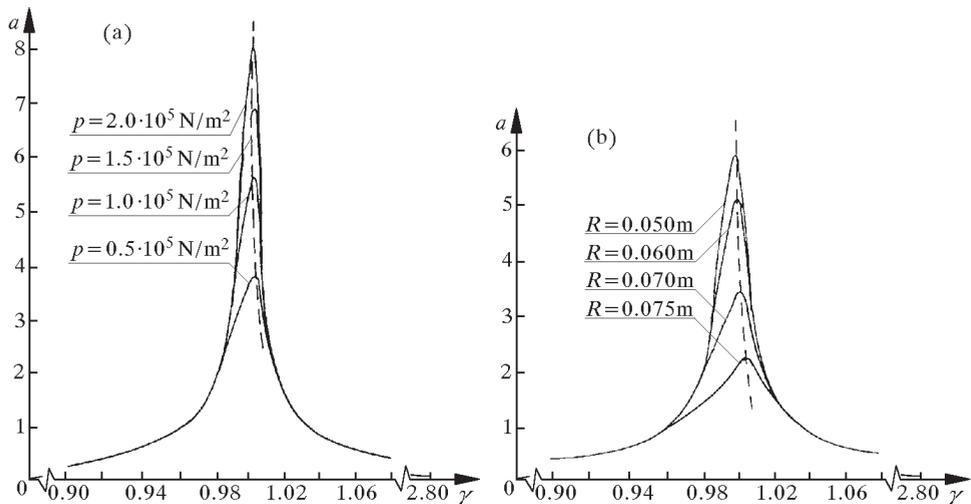
Fig. 3. Resonant curves for various values: (a) of the unit pressure  $p$ , (b) of the external radius  $R$
