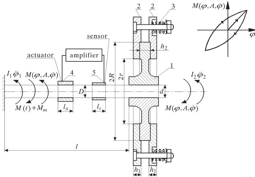
Fig. 1. Physical model of the considered friction torsional damper
