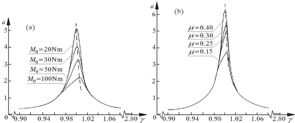
Fig. 2. Resonant curves for various values: (a) of the excitation torque amplitude  $M_0$ , (b) of the friction coefficient  $\mu$
