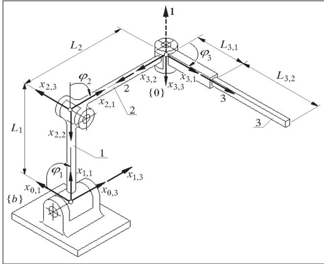
Fig. 4. Model of the manipulator
