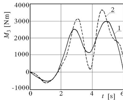
Fig. 6. Torque in the third joint required for realisation of motion; 1 – rigid link, 2 – flexible link
