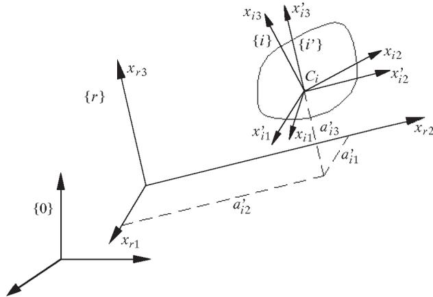
Fig. 1. Co-ordinate systems:  $\{0\}$  – inertial system,  $\{r\}$  – system connected with the moving base,  $\{i'\}$  – local system connected with the  $rfe_i$  before deformation of the link
