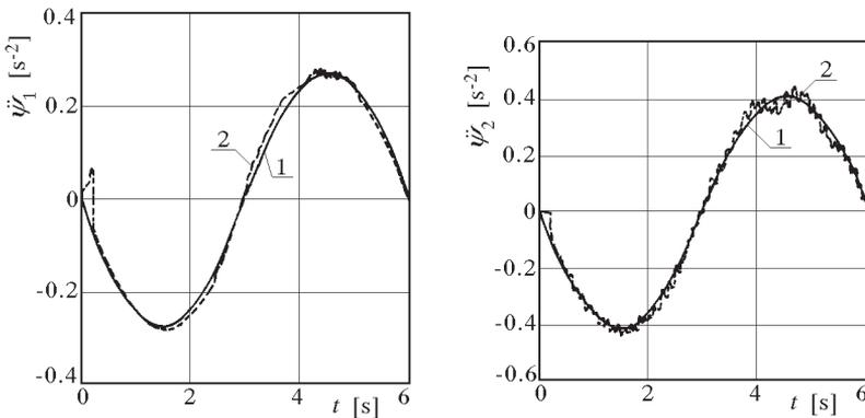
Fig. 8. Accelerations in the first and second joint, respectively; 1 – kinematic input, 2 – force input
