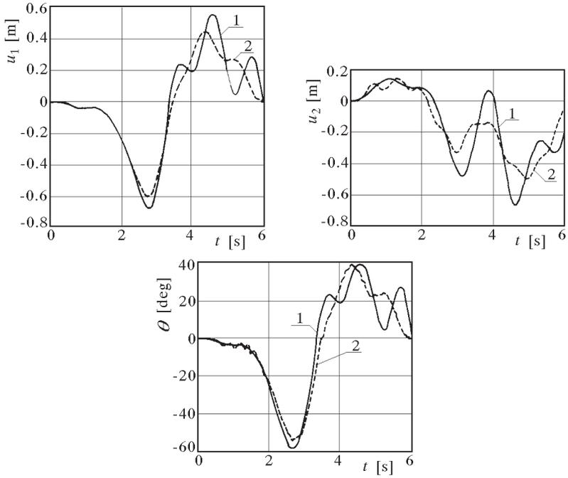
Fig. 5. Deflections  $u_1$ ,  $u_2$  and rotation  $\theta$  of the end of the third link; 1 – kinematic input, 2 – force input
