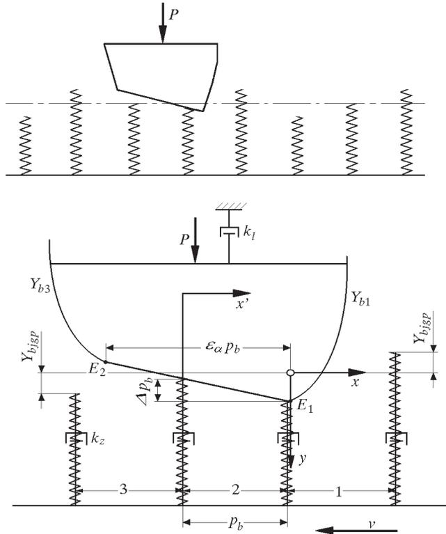
Fig. 1. One-mass, two-parameter model of gearbox by Müller (1979), where  $k_z$  – gearing’s stiffness,  $k_l$  – bearing’s stiffness,  $\epsilon_\alpha$  – tooth contact index,  $Y_{b1}$  – input tooth contact ordinate,  $Y_{b3}$  – output tooth contact ordinate,  $p_b$  – gear base pitch,  $\Delta p_e$  – gear base pitch error,  $Y_{bjgp}$  – gear pitch error,  $v$  – pitch line velocity,  $P$  – intertooth force
