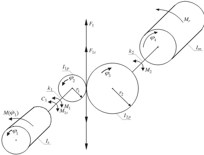
Fig. 3. System with one-stage gearbox
