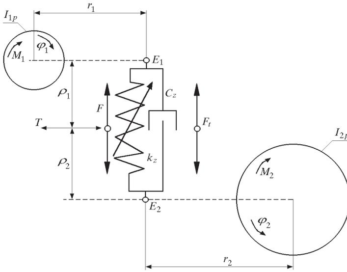
Fig. 2. Two-wheel, two-parameter model of gearbox
