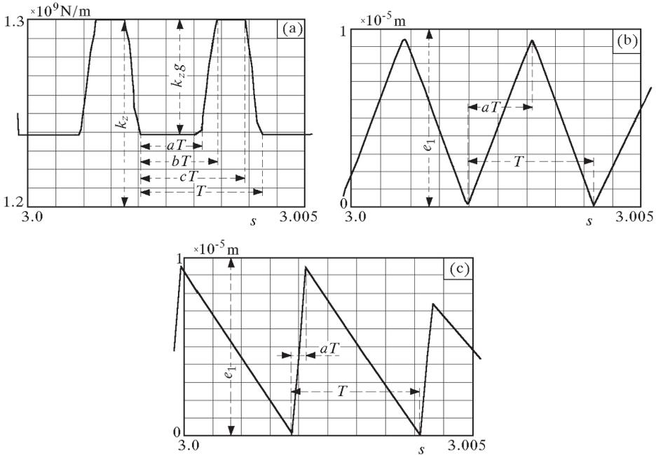
Fig. 4. (a) Stiffness function for gearing, (b) error function for error mode  $E(0.5, 10, 0.3)$ , (c) error function for error mode  $E(0.1, 10, 0.3)$
