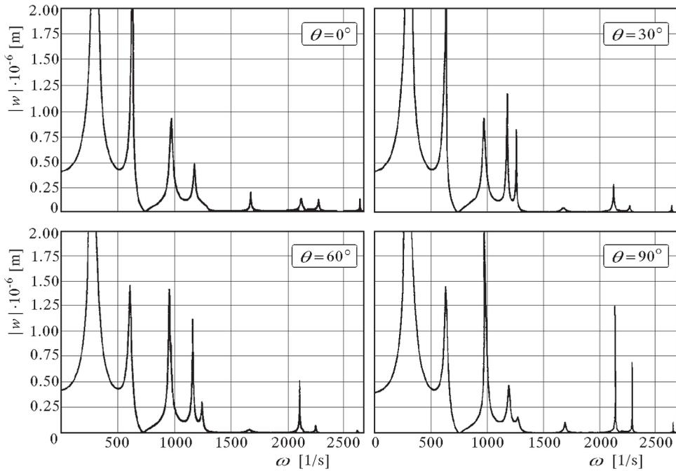
Fig. 3. Effects of variations in the skew angle on the active damping efficiency (external loading over the limited area)
