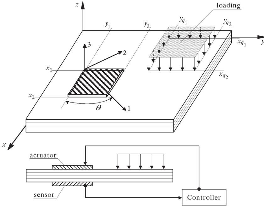
Fig. 1. Model of a laminated plate with the control device and a field of excitation
