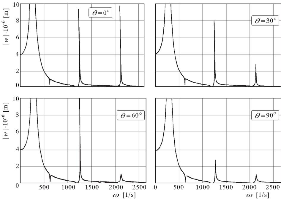
Fig. 4. Effects of variations in the skew angle on the active damping efficiency (external loading over the entire plate)
