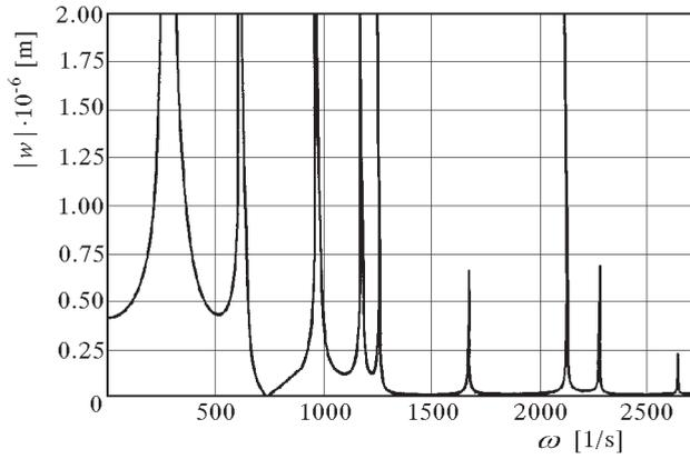
Fig. 2. Uncontrolled dynamic response in a wide range of harmonic excitation
