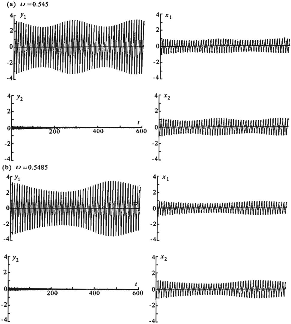
Fig. 6. Vibration time courses in generalized and quasi-normal coordinates; resonance with respect to the frequency  $p_1$
