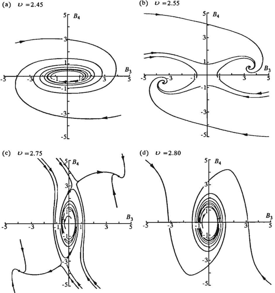
Fig. 12. Integral curves on Hayashi's surface; the main parametric resonance with respect to the  $p_2$  frequency
