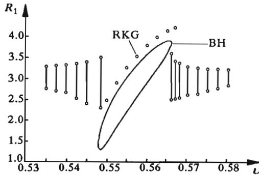
Fig. 2. Vibration amplitudes with respect to the frequency  $p_1$ , main parametric resonance, RKG method, BH-analytical investigation
