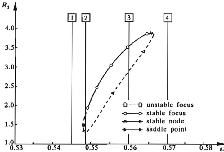
Fig. 4. Vibration amplitudes for the main parametric resonance with respect to the frequency  $\nu_1$  with the stability type marked out
