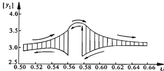
Fig. 3. Vibration amplitudes with respect to the frequency  $p_1$ , analog simulation
