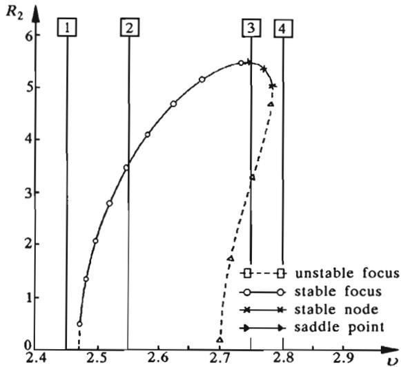
Fig. 11. Vibration amplitudes for the main parametric resonance with respect to the frequency  $p_2$  with marked stability type
