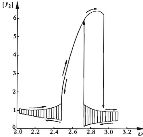
Fig. 10. Vibration amplitudes with respect to the frequency  $p_2$ ; analog simulation
