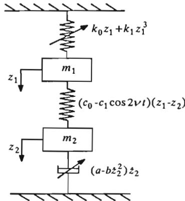
Fig. 1. Physical model of a parametrically-self-excited system with two degrees of freedom
