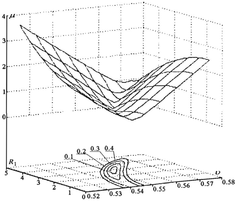
Fig. 8.  $\mu(R_1, \nu)$  chart for the resonance with respect to the frequency  $p_1$  with the contour lines for  $\mu = 0.1, 0.2, 0.3, 0.4$
