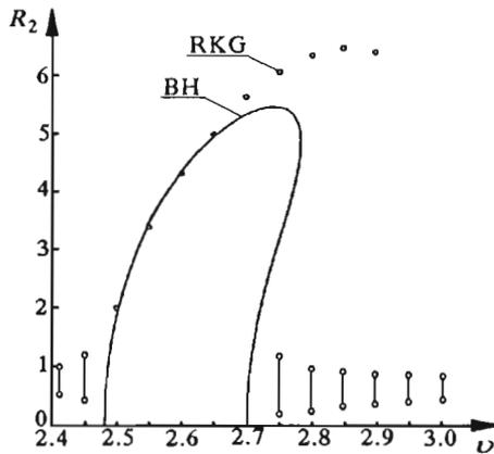
Fig. 9. Vibration amplitudes with respect to the frequency  $p_2$ ; the main parametric resonance; BH-analytical research
