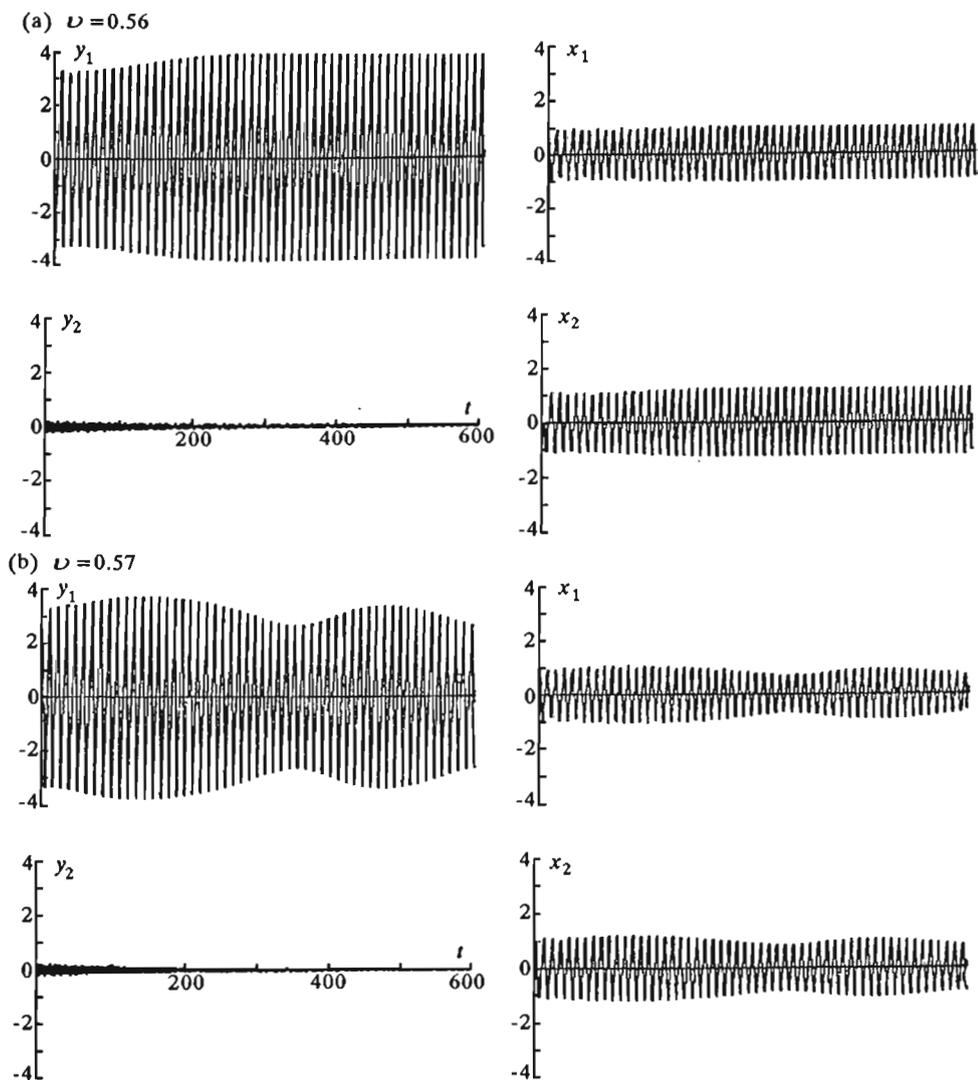
Fig. 7. Vibration time courses in generalized and quasi-normal coordinates; resonance with respect to the frequency  $p_1$
