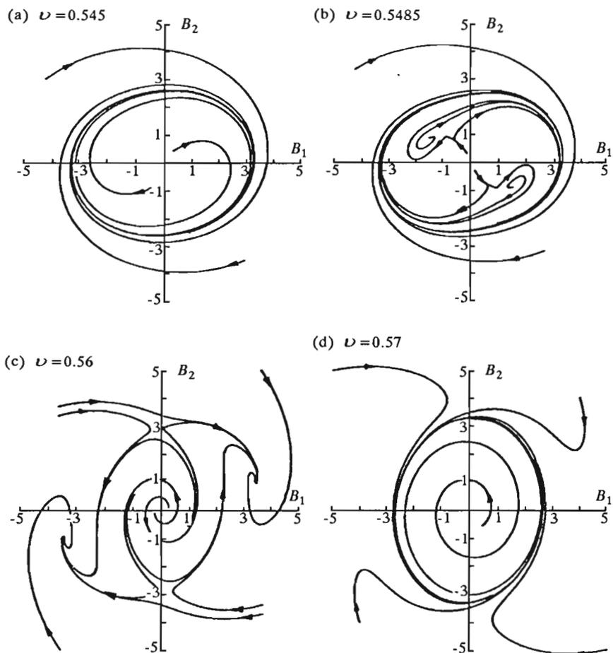
Fig. 5. Integral curves on Hayashi's surface; main parametric resonance with respect to frequency  $p_1$
