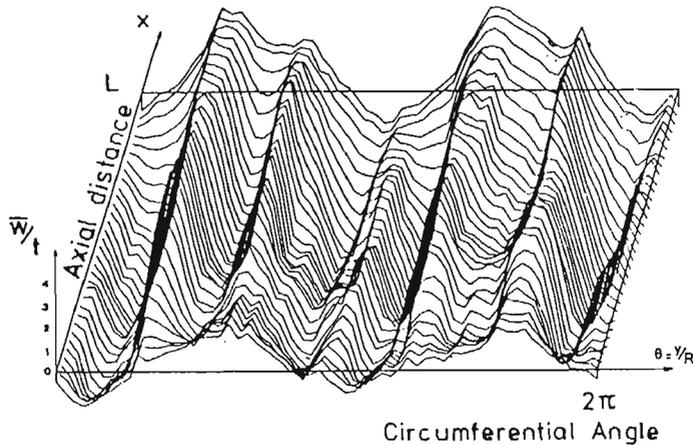
Fig. 9. Measured initial shape of Horton's shell HO-1 [15].
