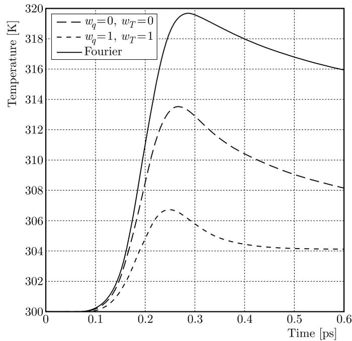
Fig. 2. Temperature history at the irradiated surface for different models (gold)
