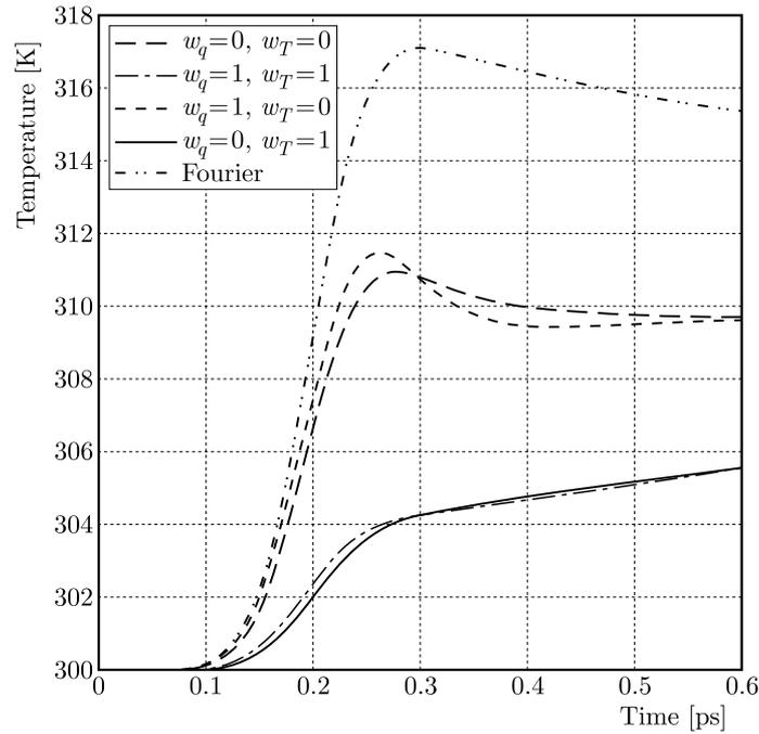
Fig. 1. Temperature history at the irradiated surface for different models (chromium)
