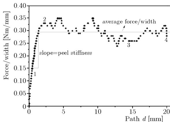
Fig. 4. The force/width vs the path curve obtained on the basis of the peeling test for interface No. 2 in the axial direction with the marked method of determining the mechanical properties, i.e. the stiffness ( $k$ ) and the average value of the force in relation to the width of the specimen ( $F/W$ ) during dissection
