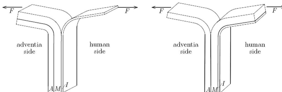
Fig. 3. Schematic illustration of the peeling test: (a) for interface No. 1 and (b) for interface No. 2. The letters  $A$ ,  $M$ , and  $I$  mark layers of the vessel wall:  $A$  – adventitia,  $M$  – media, and  $I$  – intima
