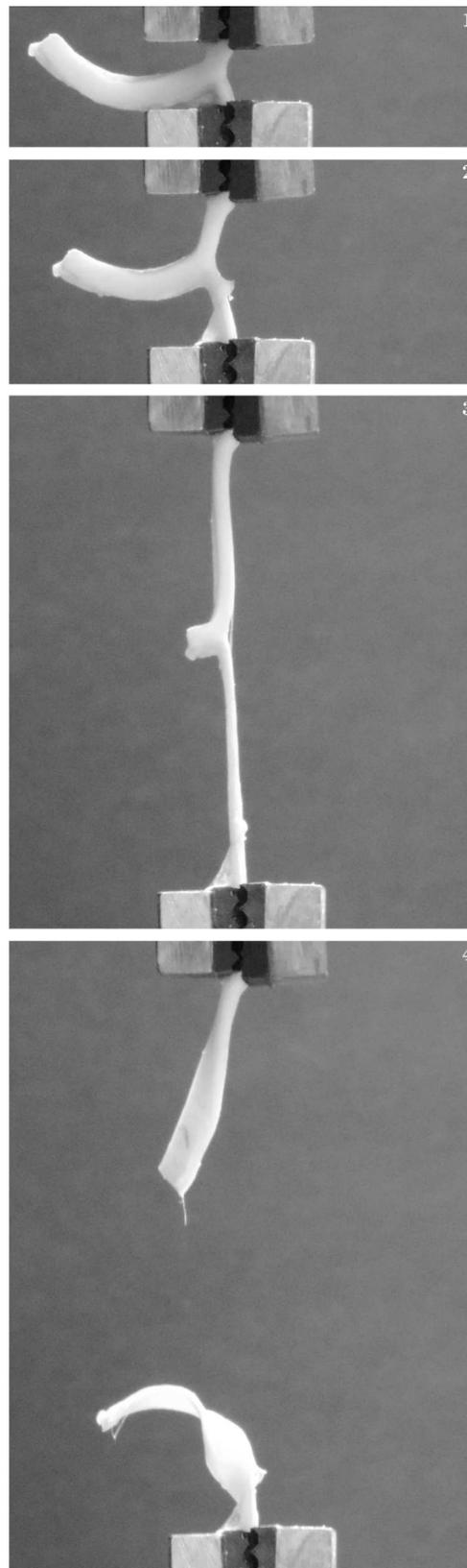
Fig. 5. Axial specimen of the arterial wall (interface No. 2) tested in the T-peel test configuration; four images (1,2,3,4) show progression of the peel test until complete separation of the tissue (4). Examples of where each image (1-4) could fall on the force/width vs path curve (Fig. 4) are indicated by numbers 1, 2, 3, and 4
