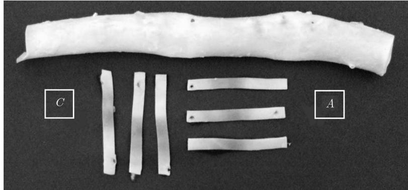
Fig. 1. Directions of specimen preparation: axial ( $A$ ) and circumferential ( $C$ )
