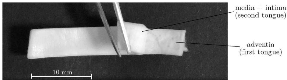
Fig. 2. Preparation of the material for tests of the mechanical properties – initial dissection of the axial specimen of the vessel wall. Width was measured for each specimen
